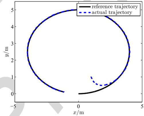
Fig. 9. Actual and reference trajectories in  $xy$ -plane under time-variant disturbances.
