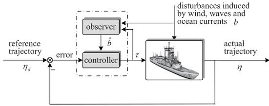
Fig. 2. Diagram of the trajectory tracking control system of a ship.
