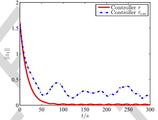
Fig. 14. Comparison of tracking performance under time-variant disturbances.
