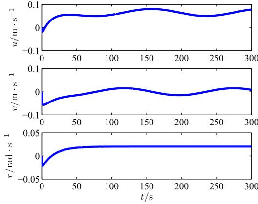
Fig. 6. Surge velocity  $u$ , sway velocity  $v$ , and yaw rate  $r$  under constant disturbances.
