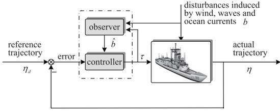
Fig. 2. Diagram of the trajectory tracking control system of a ship.
