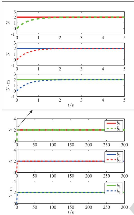
Fig. 3. Constant external disturbances  $b_1, b_2, b_3$  and their estimations  $\hat{b}_1, \hat{b}_2, \hat{b}_3$ .
