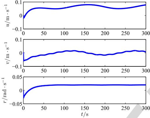
Fig. 11. Surge velocity  $u$ , sway velocity  $v$ , and yaw rate  $r$  under time-variant disturbances.
