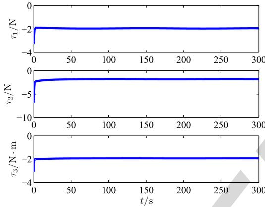
Fig. 7. Surge control force  $\tau_1$ , sway control force  $\tau_2$ , and yaw control torque  $\tau_3$  under constant disturbances.
