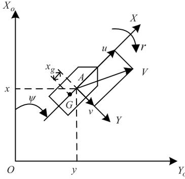
Fig. 1. Definition of the earth-fixed  $OX_oY_o$  and the body-fixed  $AXY$  coordinate frames.
