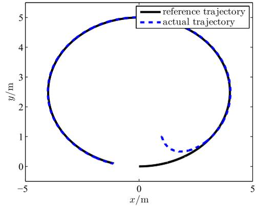
Fig. 4. Actual and reference trajectories in  $xy$ -plane under constant disturbances.
