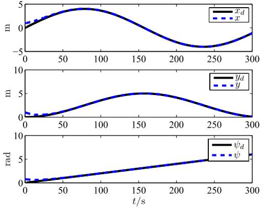
Fig. 10. Desired and actual positions and yaw angles under time-variant disturbances.
